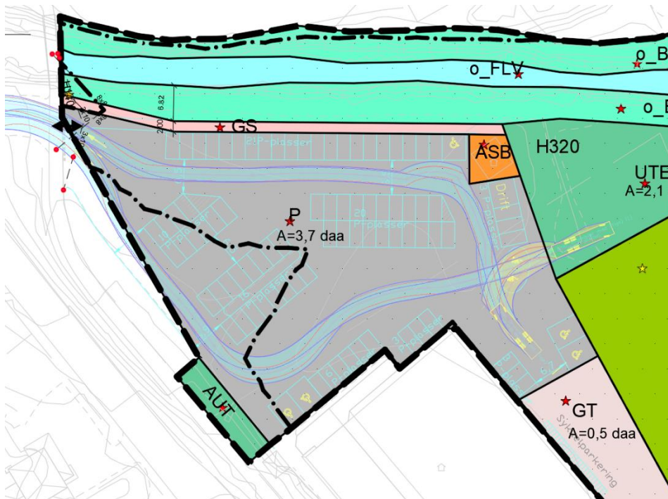
Figur 8 Sporing viser adkomst for brannbil
